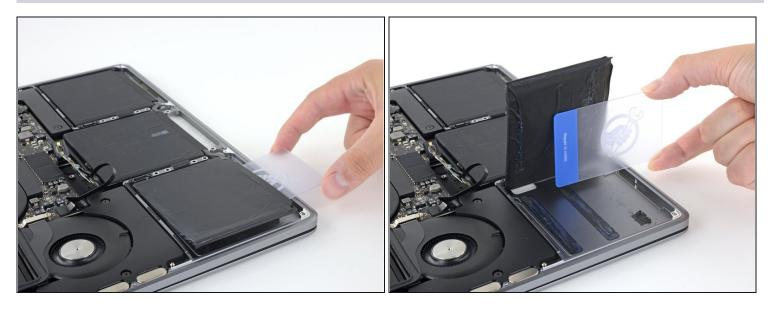
• Twist the card to raise the battery cell until it fully separates from the aluminum case.
