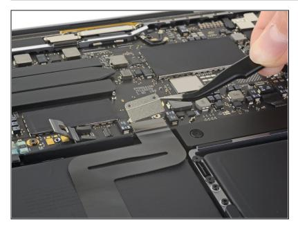
• Remove the trackpad cable connector bracket.
