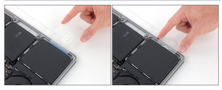
• Gently work the card deeper under the battery cell to break up the adhesive securing it in place.
