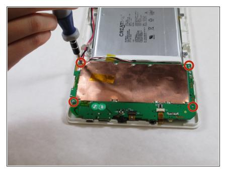
Remove the four 4mm Philips #00 screws on the edges of the circuit board.
