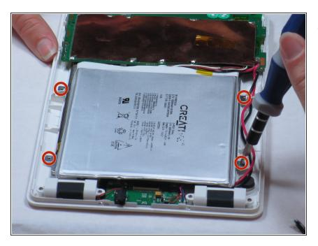
Remove the four 3mm Philips #00 screws around the large silver battery.
