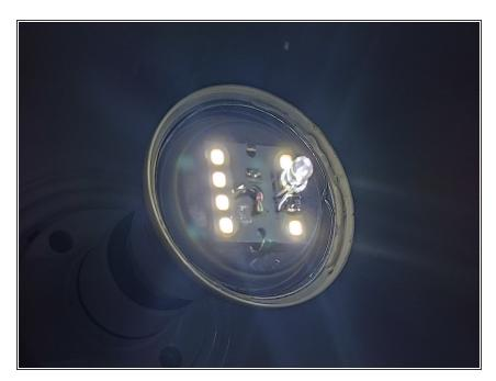
Connect the bulb to a power source to detect if it's working.
