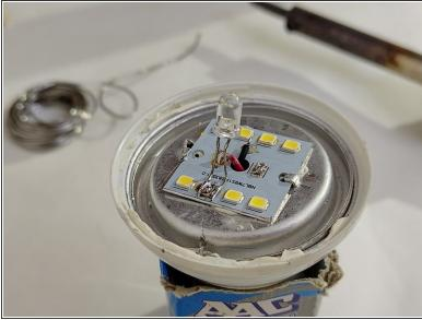
• Using the soldering iron solder an LED or a  $100\Omega$  (2W or 5W) resistor into the faulty LED space.
