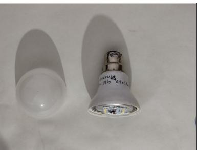
Remove the upper semi-sphere diffuser by twisting or applying some heat with a heat gun or dryer to soften the adhesive.
