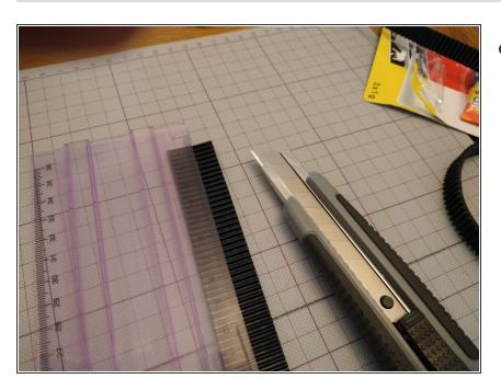
Using a sharp knife and a straightedge, cut the belt to the desired width.
