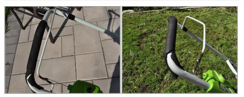
As seen in the picture, the lever is snapped on one side of the lever and needs replacement.
