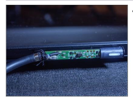
Test that the adapter is working again before closing the connector. The white LED should turn on when plugged in your Surface Pro
