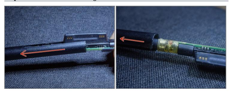
• Slide the outer case of the connector towards the cable side to uncover the connector
