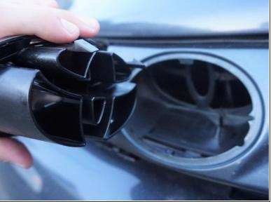
Before inserting the car emblem into the notch, be sure to align the emblem with the notch's grooves.
