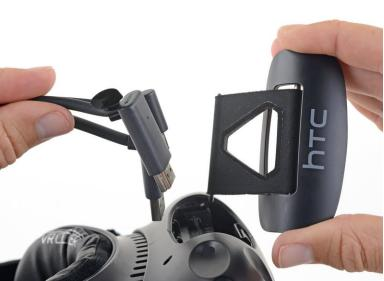
Carefully slide the compartment cover assembly over the plugs and remove it.
