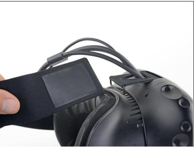
• Slide the top part of the head strap through its metal loop on the headset to remove it.
