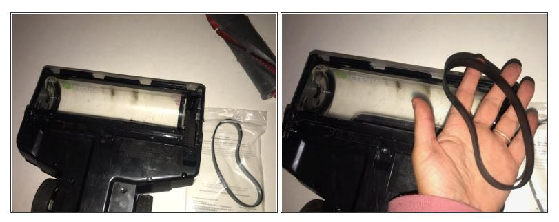
• Slide the vacuum belt out from beneath the wheel holding it in place.
