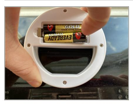
Remove the bottom battery by using your nail to lift and push toward the spring. Once the battery is lifted, remove it and set aside.
