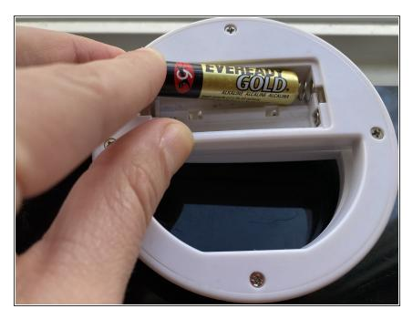
• Insert the first new battery on an angle with the negative end first so that it is pressed up against the spring. This will allow you to push the spring until it is flattened, and then push the positive end downward into position.
