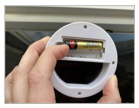
Remove the top battery in the same manner, using your nail to lift the end that is not against the spring, and push against the spring with the battery until battery is able to be lifted and pulled out.
