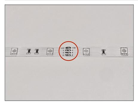
• Find the spot where the lights stop working and where there are four connections labeled in descending order, "12V, R, G, B" with a scissor "cut here" marking and a copper colored backing.
