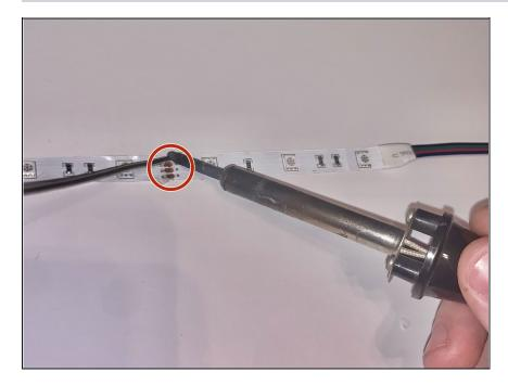
Align the new strip next to the working strip and keep them steady. Look at the four connections like a mirror image. R to R, G to G, and so on and so forth. Apply solder in any order for all four connections. Make sure solder is secured and steady.
