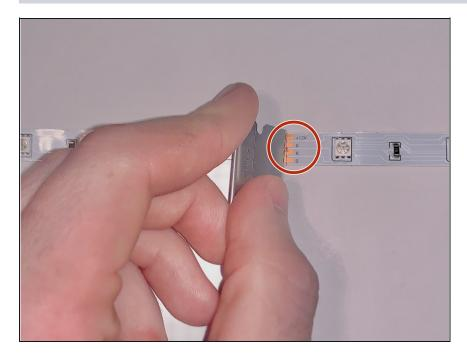
• With a scissor, cut along the "cut here" line, separating the faulty strip from the working strip.
