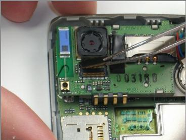
• Locate the camera near the upper-left corner and use the metal <u>tweezers</u> to carefully detach the black tab.
