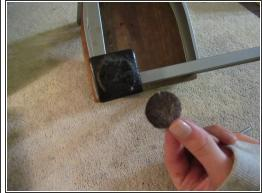
Using an Exact-o knife or boxcutting blade, carefully cut away the worn out felt footing.
