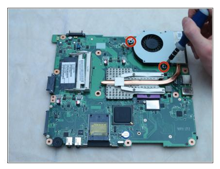
Flip the motherboard over. Remove the two 3-mm screws from the fan using a Phillips #1 screwdriver.
