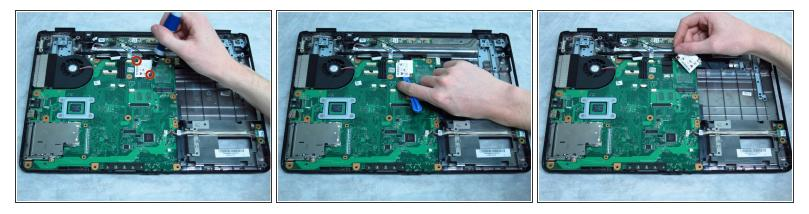
Remove the two 3-mm screws from the card connected to the black wire using a Phillips #00 screwdriver.
