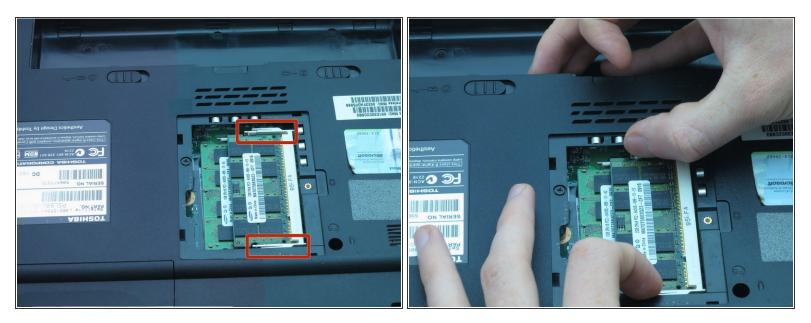
Push the white and silver retaining clips away from each side of the RAM card using your fingernails.
