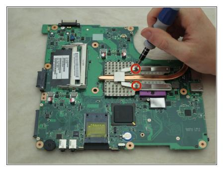
Using a Phillips #1 screwdriver, remove the two 3-mm screws locking the heat sink in place.
