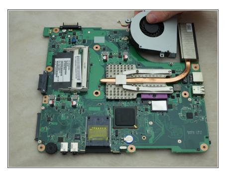
• Remove the fan from the heatsink using your fingers.
