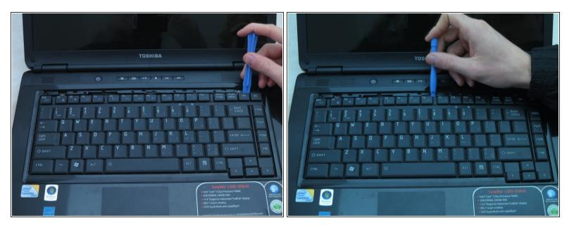
• Pry the top of the keyboard loose from its casing using a plastic opening tool.
