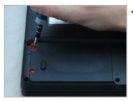
Loosen the two captive screws on the bottom left corner of the hard drive using a Phillips #1 screwdriver until you hear a click.
