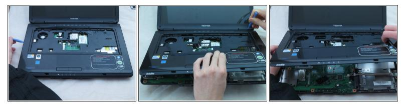
Separate the laptop upper casing from the lower casing by using an opening tool around the sides of the case to pry it apart.
