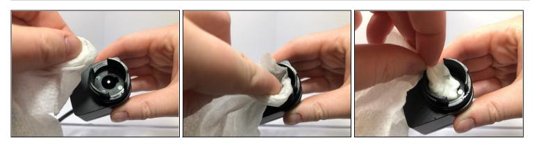
Wipe the shaft and the cavity with a damp paper towel to remove vinegar.
