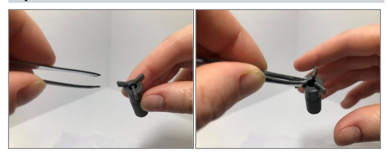
• Pick up the new impeller using tweezers.
