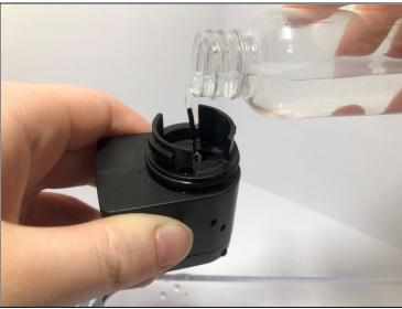
• Fill the impeller cavity with water.
