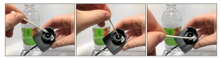
• Clean the shaft and the cavity with Q-tips dipped in vinegar in a scraping motion.
