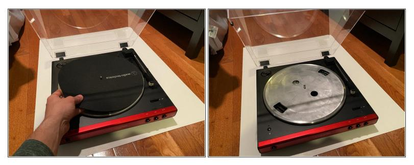
• Remove the felt pad, and put it to the side.
