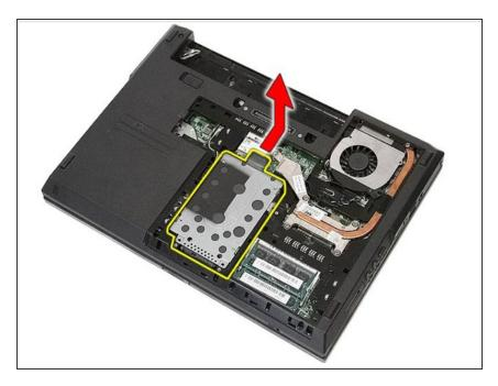
Slide the hard drive towards the center of the computer and remove.
