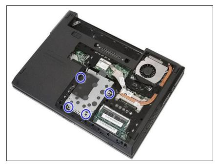
Locate and move the screws securing the hard drive to the computer.
