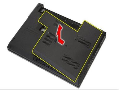
After removing the battery., loosen the screw(s) that secures the access panel to the computer, then that secures the access panel to the computer.
