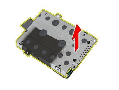
Remove the screws securing the hard drive caddy to the hard drive. Then, lift up the hard drive caddy at an angle from the hard drive and remove.
