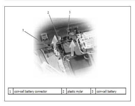
Remove the coin-cell battery connector from the connector on the system board.
