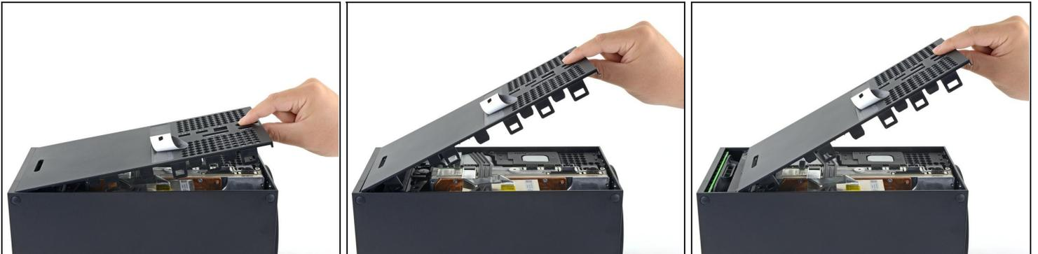
The back panel slots into a gap at the top of the shell.
