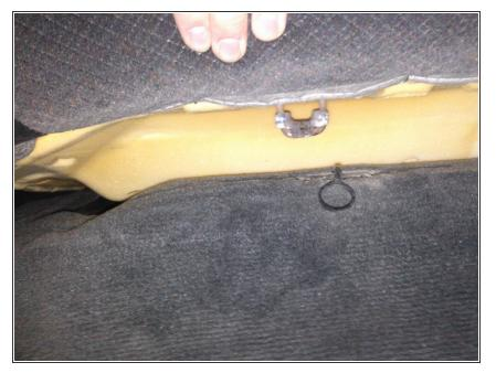
• Lift up and remove the seat.
