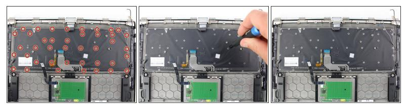
• Remove the forty-one 1.9 mm screws from the keyboard panel with a Phillips #000 screwdriver.
