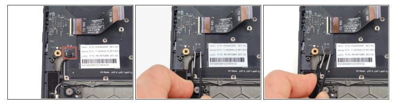
Use a pair of blunt nose tweezers to pull out the speaker cable on the lower portion of the daughterboard.
