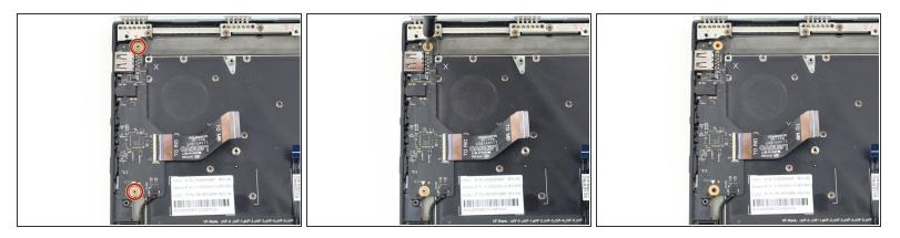
Use a Phillips #00 screwdriver to remove the two 3.6 mm screws from the daughterboard on the left.
