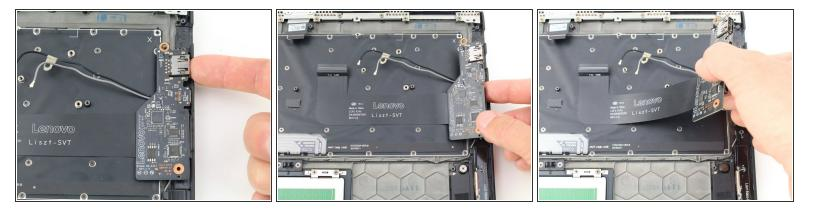
Lift the daughterboard from the right edge and peel off the interconnect cable from the keyboard panel.
