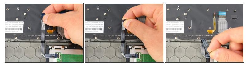
• Peel back the trackpad cable from the black keyboard panel.
