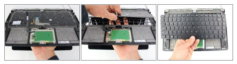
• Press the keyboard up from the underside and grab it to remove it from the case.
