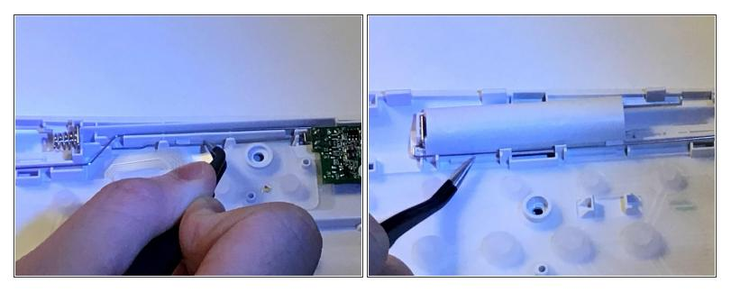
• Use a pair of tweezers to bring the metal rods under and over the plastic hooks.
