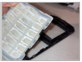
Now, pull up on the top of the board, use tweezers to push the bottom right clip in, and then pull the board to the right and up. Next, remove the fake keypad.
