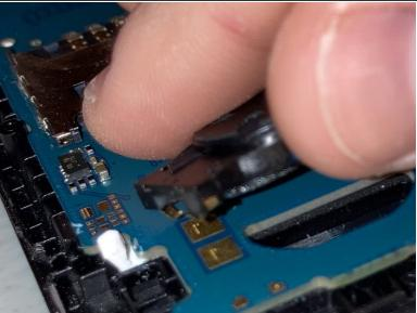
On the back of the phone, we can remove the vibration motor and then on the circuit board, you can remove the speaker.
