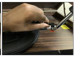
Insert a prying tool into the stylus casing, right above the red casing.
