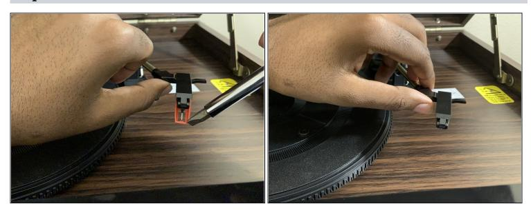
• Push the casing down with the prying tool, releasing it so it can be removed.
