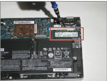
• Use a Phillips #00 screwdriver to remove the single 3 mm screw on the right of the SSD.
