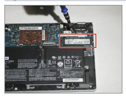
Disconnect and pull the SSD out of the motherboard.
