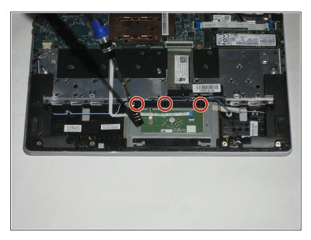
Using a Phillips #00 screwdriver, remove the three 3mm screws located at the top of the trackpad.
