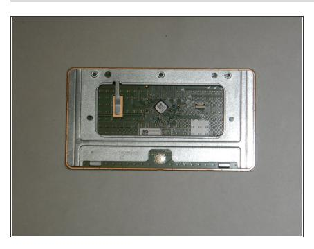
• Remove the trackpad from the device.
