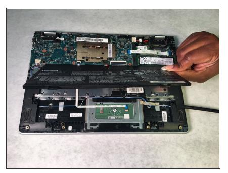
Remove the battery carefully from the device by lifting up the edge nearest you and then gently pull toward you to disconnect the power wires.
