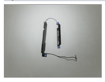
Remove the speakers from the device.
