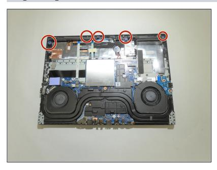
Remove the five screws using the Phillips #0 screwdriver.
