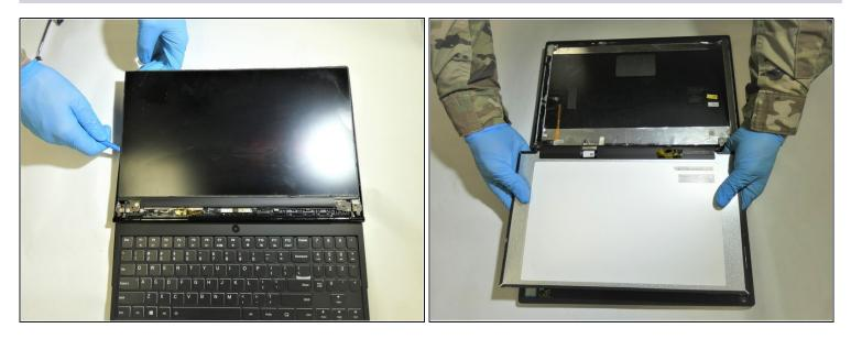
• Carefully insert the plastic opening tool behind the screen to remove the adhesive.
