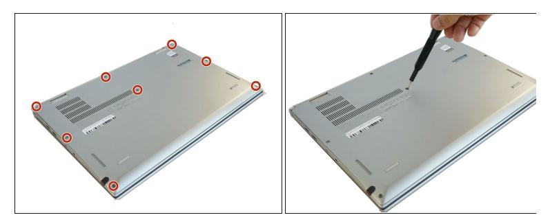
• Use a Phillips #0 screwdriver to remove the eight 8 mm screws.
