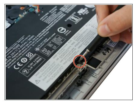
• Use a Phillips #0 screwdriver to remove one 6 mm screw from the bottom-middle portion of the battery.
