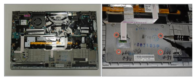
Using a Phillips #0 screwdriver, remove four 3 mm screws.
