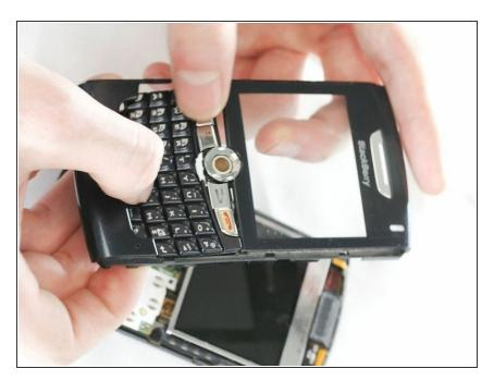
• After removing the front from the outer casing, the track ball will come off attached to the casing.
