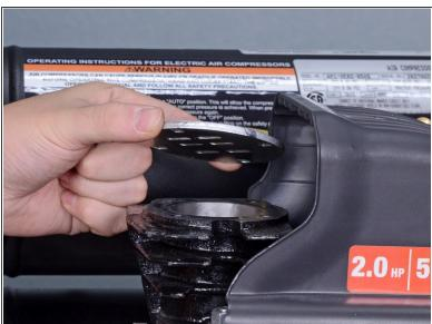
Remove the lower valve plate.
