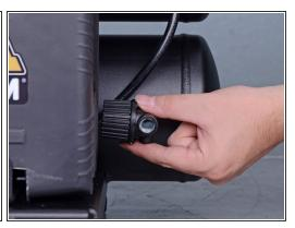
Rotate the regulator 180°, so the bottom of the regulator faces away from the compressor motor.
