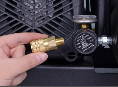
Use a 3/4 inch wrench to loosen and remove the air hose quick-connect socket.
