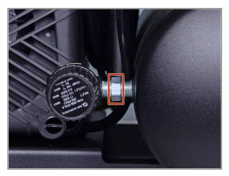
Use a 5/8" wrench to loosen the air tank nipple from the air tank enough to be able to rotate it with the regulator.
