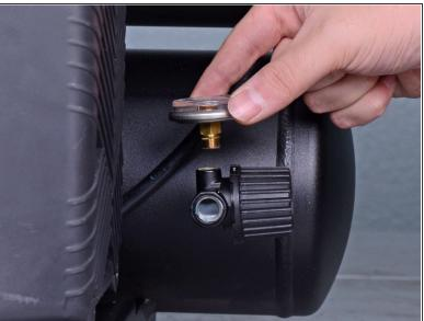
Use a 7/16 inch wrench to loosen and remove the pressure gauge.
