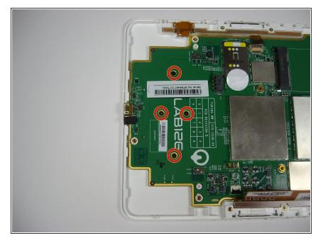
Use a Phillips #00 screwdriver to remove the four 4 mm screws from the motherboard located around the LAB126 logo.
