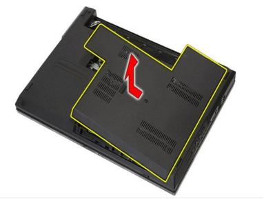
• After removing the battery, loosen the screw that secures the access panel to the computer. Then, lift up the access panel at an angle and remove it from the computer.
