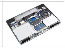
After removing the battery, remove the screws securing the access panel in place. Then, lift the top edge of the access panel upward and remove the access panel.
