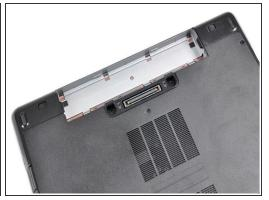
Slide the battery release latches into the unlock position. Then, rotate the outer edge of the battery upward and remove from the system.
