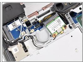
• After removing the access panel, locate the CMOS battery in the mid-left section of the panel. Careful disconnect the CMOS battery cable from the system, then pry the CMOS battery upward to remove. NOTE: Remember not to touch any of the system components when the panel is open, as doing so could damage your system via electrostatic discharge.
