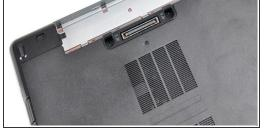
Slide the battery release latches into the unlock position. Then, rotate the outer edge of the battery upward and remove from the system.
