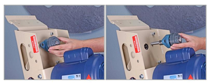
• Remove the cam shaft assembly
