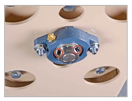
Use a 1/8 inch hex key to loosen the two set screws on the lower flange bearing.
