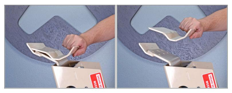
• Remove the blade retainer.
