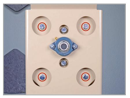
Use a 9/16 inch socket to remove the four bolts securing the striker plate to the isolators.
