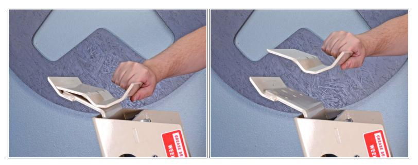
• Remove the blade retainer.
