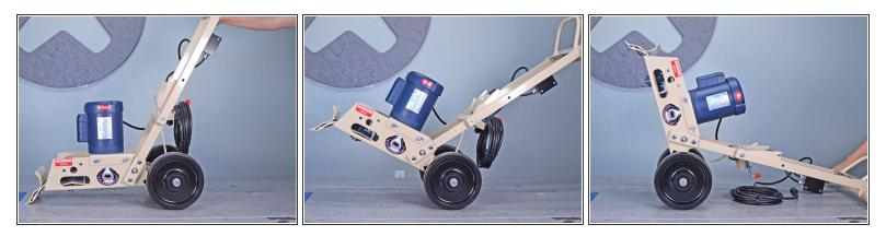
• Tilt the device back to rest on its handle.
