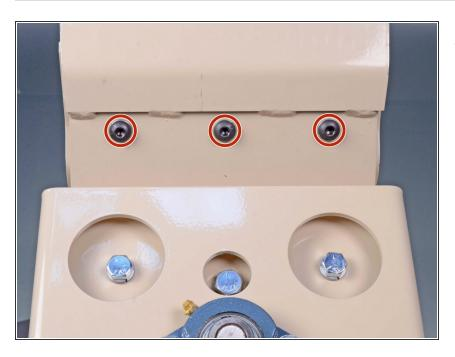
Use a 3/16 inch hex key to remove the three bolts securing the blade retainer.
