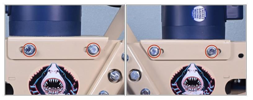
Use a 9/16 inch socket to loosen, but not remove, the four bolts securing the motor mount to the frame, two on each side.
