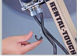
Remove the loom clamp from the power cable.
