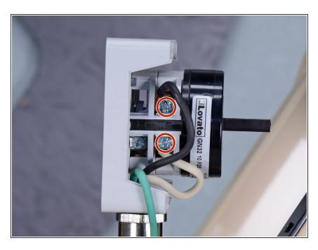
Use a flathead screwdriver to loosen the two screws securing the wiring harness's black and white wires to the switch.
