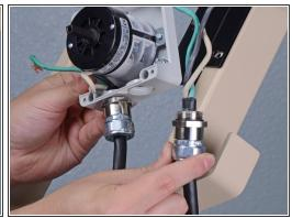
Remove the power cord from the on/off switch.
