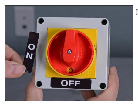
Reassembly tip: ensure the replacement switch is labeled with the correct stickers, matching the old part."
