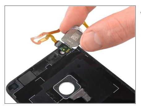
Remove the fingerprint sensor.
