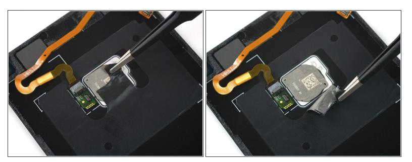
Peel off the black sticker until the sensor is completely exposed.
