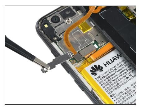
Use a pair of tweezers to remove the metal shield.
