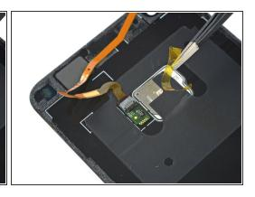
Use a pair of tweezers to peel off the yellow protective sticker from the fingerprint sensor connector.
