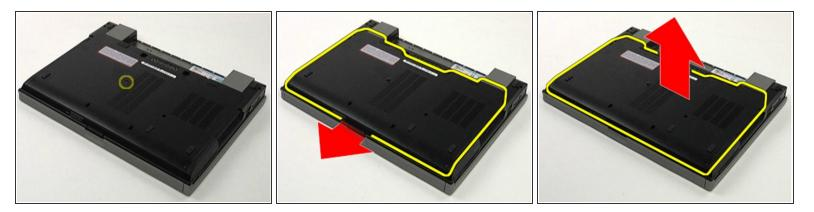
• To remove the access panel, use your screwdriver to remove the single screw in the center of the base. Then, slide the access panel toward the front of the system and lift it from the system.
