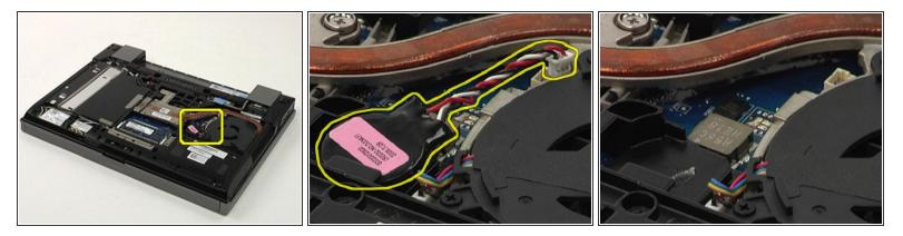
• After removing the access panel, locate the coin cell battery. Then disconnect the battery cable from the system board and lift the coin-cell battery out of its socket to remove.
