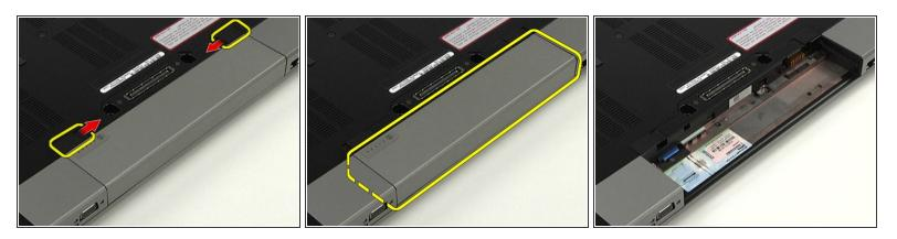
• To remove the battery, slide the latches inward, and remove the battery from the system.
