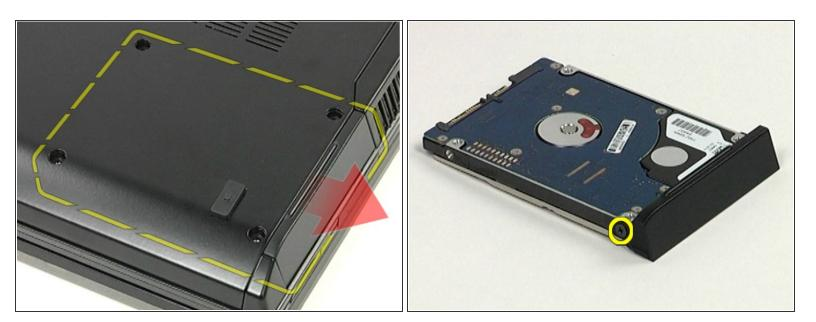
Slide the hard drive out of the laptop. DO NOT TOUCH THE COMPONENTS OF THE DRIVE.
