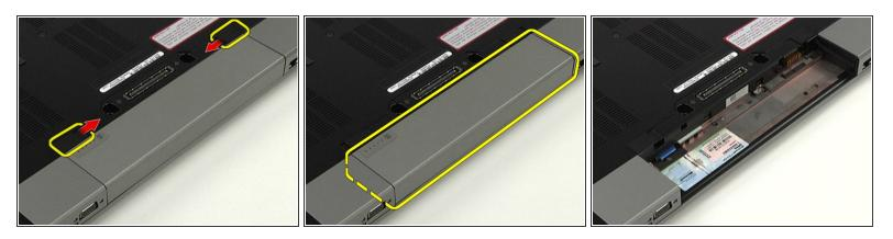
Slide the latches on the battery and remove the battery.
