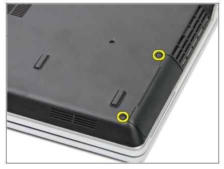
Use a Phillips screwdriver to remove to the screws that secure the hard drive from the hard drive caddy.
