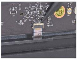
• Use the pointed end of a spudger, an opening tool, or your fingernail to flip down the small, hinged locking flap on the ribbon cable <u>ZIF connector</u> on the front circuit board.
