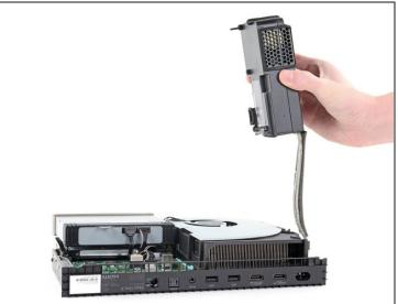
• Lift the power supply so that the cables are at a 90 degree angle.
