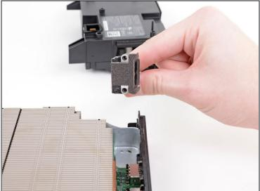
• Lift the power supply socket out of the upper metal case.
