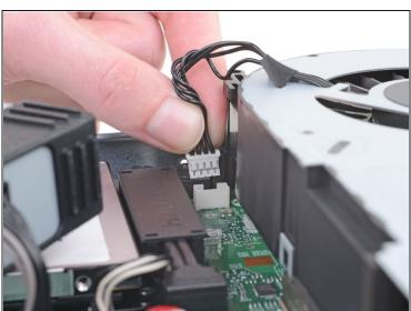
Unplug the bundled cable connector connecting the fan to the motherboard by pulling directly upward.
