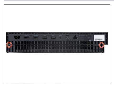
Use a T10 Torx screwdriver to remove the two 12.6 mm–long screws located on the back of the console.
