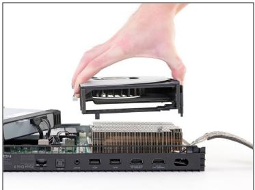
• Lift the fan case up to remove it from the console.
