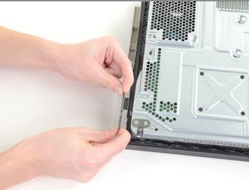
Pull the front circuit board straight out away from the upper metal case and set it aside.
