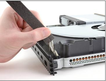
• While holding the power supply above the console, move the two grey cables out of the plastic hook on the fan case.
