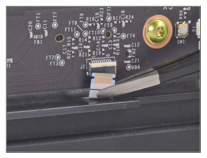
Use blunt tweezers to pull the ribbon cable down out of the connector.
