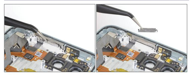
After removing the motherboard, the top spacer will usually fall out. To replace it, reposition the midframe without screwing it down. Grasp the spacer with the tweezers and compress the interior foam to squeeze it into position. Then screw the midframe into place.
