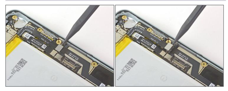
• Use the pointed end of the spudger to pry the battery connector straight up and disconnect it from the motherboard.
