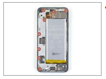
• Use a T3 Torx driver to remove the eight 4.6 mm-long screws securing the midframe.
