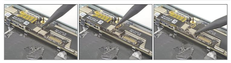
• Use the pointed end of a spudger to disconnect the two press connectors by lifting them straight up from the motherboard.
