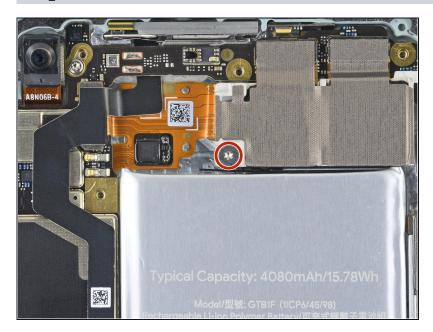
• Use a T3 Torx driver to remove the 4.1 mm shouldered screw.
