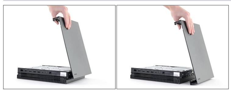
• Push the upper plastic case down and away from the console to remove it completely.
