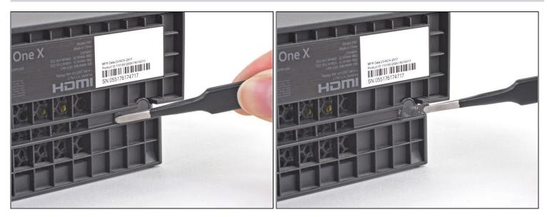
• Use blunt <u>tweezers</u> to peel off the sticker covering the right-side screw on the back of the console.
