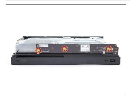
Use a T8 Torx screwdriver to remove the three 13.3 mm screws securing the front circuit board to the upper metal case.
