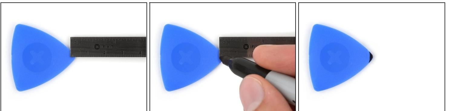
**ⓘ** If inserted too far, an opening pick can damage your device. Follow this step to mark your pick and prevent damage.
