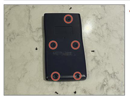
Use a Philips #0 head screwdriver to remove the five screws on the back of the device.
