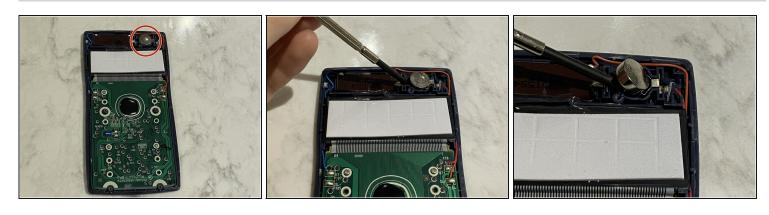
Use an opening tool to gently remove the battery from the device.
