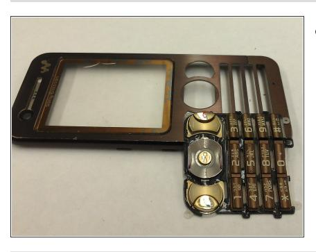
Separate the front and back panels that were pryed open with the plastic opening tool.
