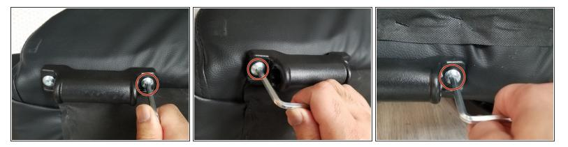
• Tighten the four 25 mm hex screws located at the bottom of the chair using the 3 mm Allen key.
